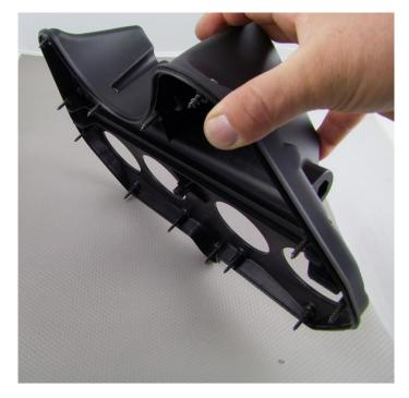
3. Remove the bottom side of the air box and then remove the stock air filter and the plastic frame.
