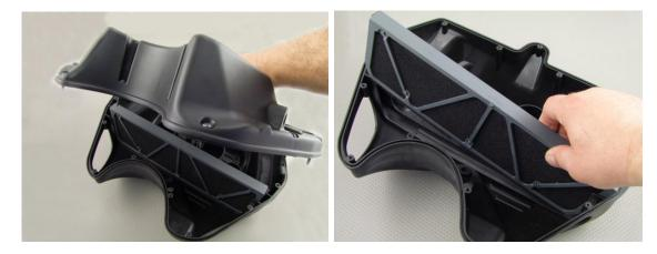
4. Clean the air box carefully and install the DNA filter. Push it firmly on the top so it sits properly in the slot.
