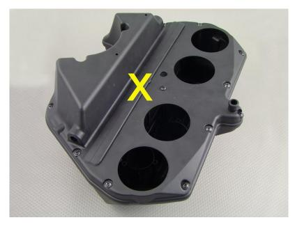
2. Unscrew all 13 screws that keep the air box assembled. DO NOT REMOVE them from the bottom part of the air box!
