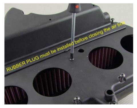
8. If the DNA air filter is installed correctly it should look as bellow.
