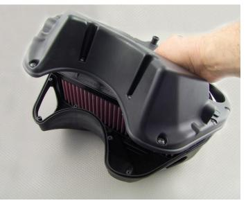
Align the 2 air box parts, check that the DNA filter is aligned with the slot, and if yes close the air box. At this point if everything is done correctly the air box will close without any force. If the air box needs force to close or it does not align, re-check and correct as necessary.
