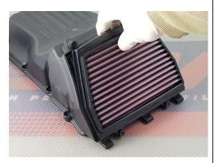
4. Place the DNA laser cut frame on top of the filter and bolt the 2 lower bolts, not completely, stop 1 mm before they tighten. Attention! At this point the frame must be loose.
