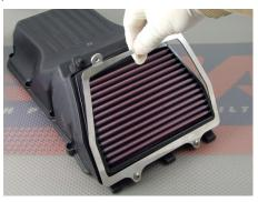
5. Bend the frame over the filter and bolt the 2 top bolts. Stop 1 mm before they tighten.
