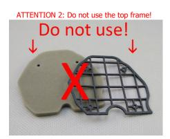
2. Install the DNA filter and close the air box cover.
