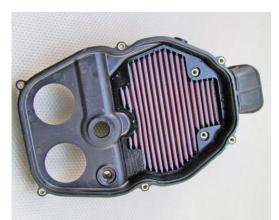
Follow the above procedure each time you need to remove the DNA filter for servicing it. Service every 15.000 km or earlier when used in extremely dusty environment.
