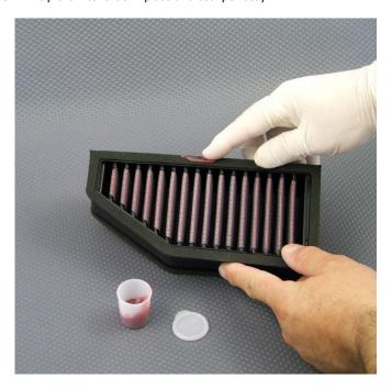
NOTE: We recommend using latex gloves to apply the DNA sealing grease.
