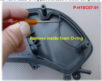
**Attention !!!**: if the foam O-ring is not removed the filter will not sit properly in the air box, the air box cover will NOT close and possible damage to the engine will occur.
