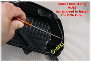
**Attention !!!** : if the foam O-ring is not removed the filter
