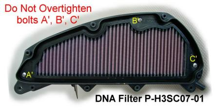
Carefully close the airbox and the installation is completed.
