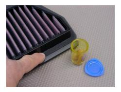
**3.** Install the DNA filter in the airbox carefully. Check that all 3 tabs are located properly in place.
