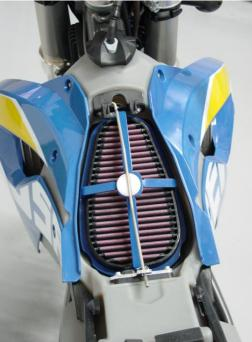
Lock the filter in place and reinstall the seat.
