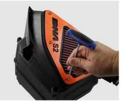
Attention! The allen bolts must be bolted under "angle" observe the position of each 'hole' before forcing the bolts and damaging the air box.
