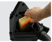
2. Install the DNA Stock replacement Air Filter P-KT6SM13-01 (SOLD SEPARATELY) in the air box carefully, push it to "sit" correctly, position the plastic retainer and secure with the 'wire' lock .
