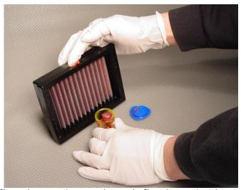
Read the information on the DNA filter and pay attention not to damage the filter when passing it between the frame and the air box during installation!
