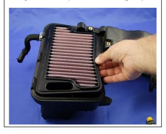
**3.** The DNA filter installed. Attention! The rubber tube is not used with the DNA filter.
