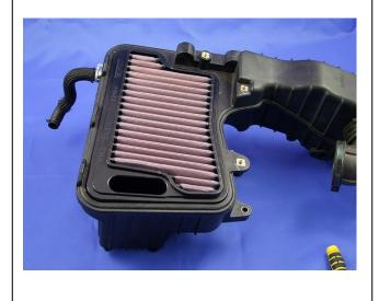
**4.** Install and close, the top air box cover, securing it with the 2 bolts.
