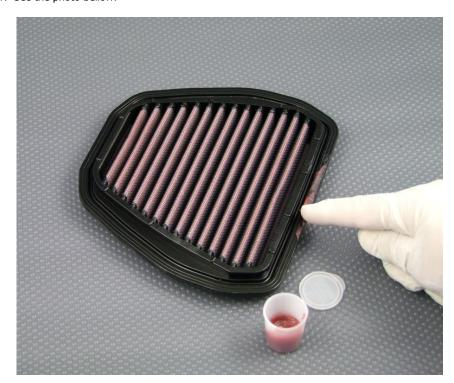
NOTE: we recommend using latex gloves to apply the sealing grease.
