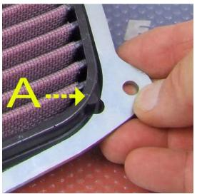
Following slide both, top frame and filter, on the bottom frame and secure using the 2 M6X16 Allen bolts supplied.
