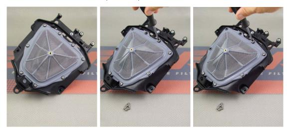
3. Remove all 8 spacers from the stock base. Attention! The 8 bolts and spacers will be used with the DNA S2 KIT
