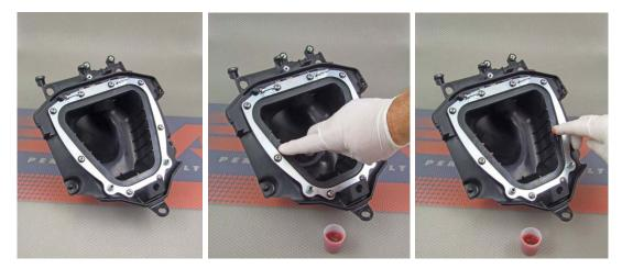
6. Install the top frame on the DNA filter. Pay attention to the locating tab of the filter, it must line up with the notch in the top frame.
