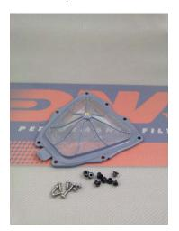
4. Apply DNA Air Filter sealing grease on the stock rubber joint where the DNA steel frame will sit. Install the frame carefully and check if it has been 'centered' with the rubber joint. Install the 8 stock spacers and then bolt the frame using the stock bolts.
