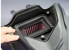
Bolt the filter frame in place; reinstall the cover and body work, following the BMW service manual.
