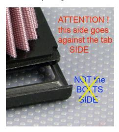
One side of the DNA filter is specially designed to seal perfectly against the TAB side of the air box. If this side is not placed correctly the filter will not sit properly in place and plastic BMW frame will be DAMAGED, dirt will enter the air box and possible engine damage will occure.
