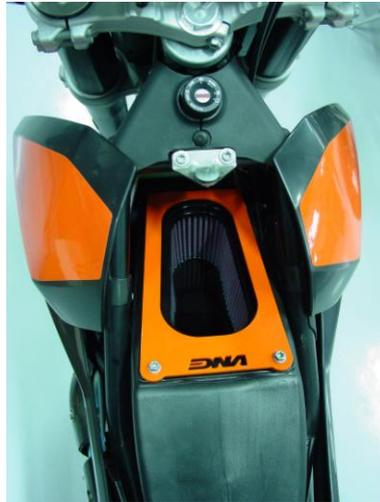
4. **Attention!** When washing the bike the air box intake must be covered, to stop the water entering the air box. If by mistake the air box is flooded, it must be cleaned and dried BEFORE starting the bike, or else damage to the engine can occur.
