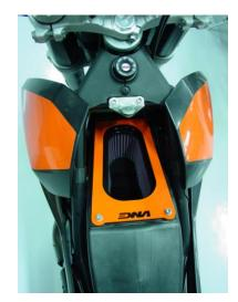
4. **Attention!** When washing the bike the air box intake must be covered, to stop the water entering the air box. If by mistake the air box is flooded, it must be cleaned and dried BEFORE starting the bike, or else damage to the engine can occur.
